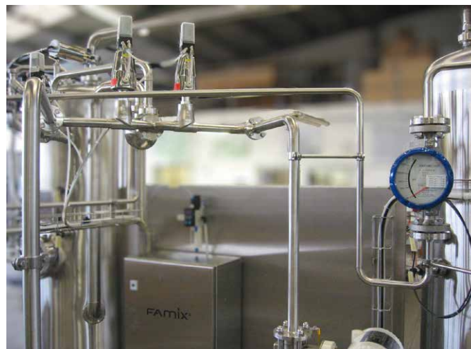
CO 2 measurement using a float. Flow meter for determining the CO 2 addition to reduce the residual O 2 value to < 0.1 mg/l.
