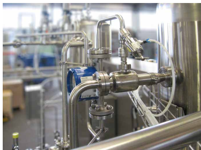
Fine adjustment for the addition of CO 2 from 0-2 g/l with carbonation unit.
